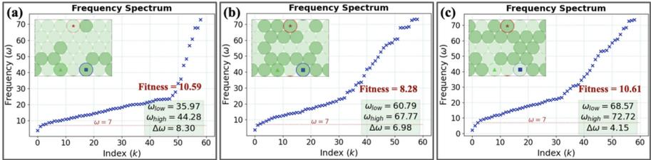
**Fig. 8.** The most “AND-like” stiffness-varying materials from the three evolutionary trials. The band gap for each configuration is shown below each of them.
