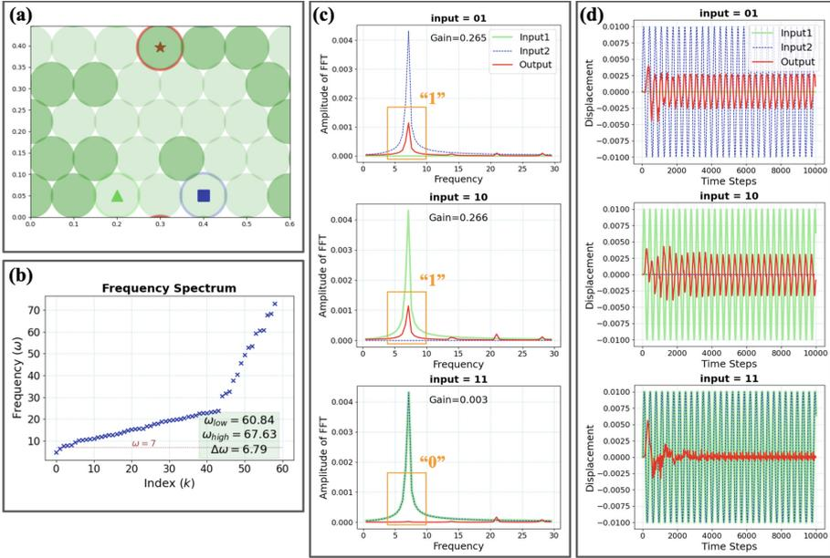
**Fig. 13.** One of the most XOR-like evolved materials, composed from stiffness-contrasting particles. (a) and (b) report the configuration and its band gap features. (c) reports how the material responds at the driving frequency (7) and all other frequencies. (d) shows how the three ports displace, over time, during three of the four input cases.
