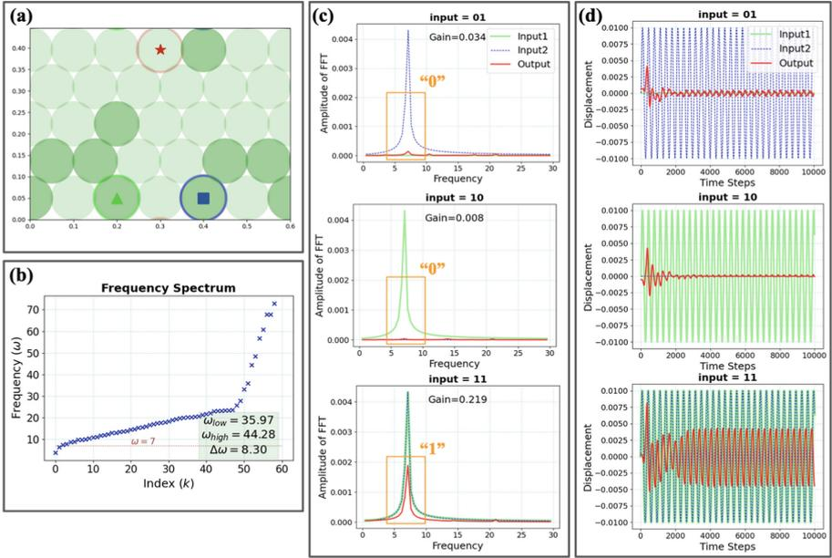
**Fig. 7.** One of the best designs for an AND gate with stiffness-contrasting particles. (a) and (b) show the configuration and its band gap respectively. (c) shows the response of the material at the driving frequency, and the other frequencies, for three of the four input cases. (d) shows the displacements of the input ports and the output port over time.
