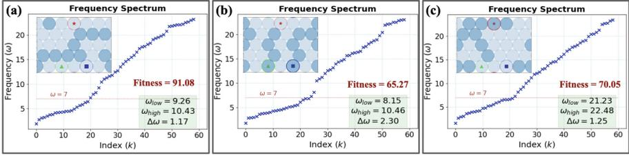
**Fig. 11.** The most XOR-like mass-varying materials found by each of the three evolutionary trials. The frequency spectrum of each configuration along with its fitness values is shown below each one.
