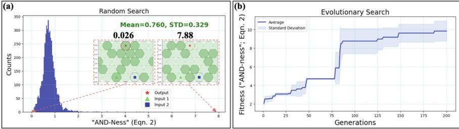
**Fig. 6.** Designing an AND gate in a stiffness-contrasting assembly of particles. (a): The histogram shows the distribution of “AND-ness” in 5000 random configurations, as well as the best and worst material found. Light and dark green colors indicate soft and stiff particles, respectively. (b): The plot shows the progress of optimization during 200 generations. (Color figure online)
