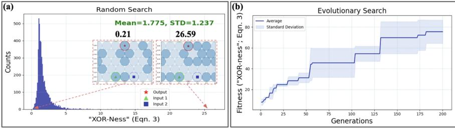
**Fig. 9.** Designing an XOR gate in a mass-contrasting assembly of particles. (a): The histogram shows the distribution of XOR-ness across 5000 materials found via random search. (b): Progress of evolutionary optimization.
